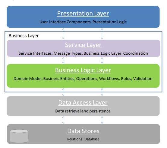
An ideally designed n-layered architecture each layer should be aware of and communicate only with the layer existing one level below. Additionally, communication should be done through well-defined interface contracts. This can be achieved by using interface-based programming. This is not always the case in practice, obviously - any design decisions depend on various factors like requirements, complexity of the application, time available, etc.
