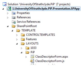
As seen in the snippet, additionally to the ClassDescriptorForm.aspx file there is a ClassDescriptorForm.js file which contains all JavaScript code needed for the purpose of user interface demonstrator. In actual fact, almost all of the user interface logic was written in Java Script and jQuery for the purpose of the demonstrator.
