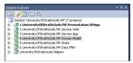
The solution consists of 7 sub-projects. Each sub-project corresponds to given layer / component of the application (solutions' names start with numbers to order them from top to bottom layers).
